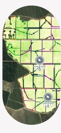
Single platform that controls and reports on all irrigation systems (developed with the know-how of our team), enabling the technicians to control and know, in real time, where and how much watering is taking place and then optimise water use and detect problems such as punctual ruptures or interruptions, being able to start or stop any of the systems remotely. This platform also optimises energy use, as it privileges irrigation during periods of greater energy availability.
